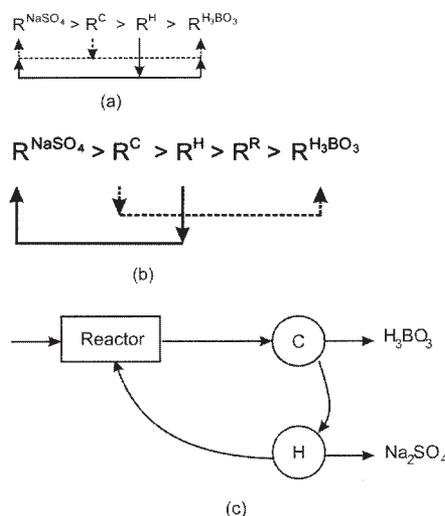
**Figure 12. Production of boric acid starting with ulexite.**
