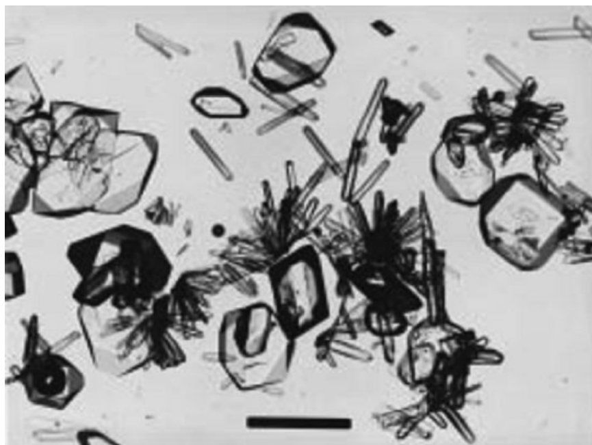
Figure 2. Solution mediated conversion of orthorhombic paracetamol to monoclinic paracetamol in benzyl alcohol. The scale bar represents 250 \mu\text{m} . 21
