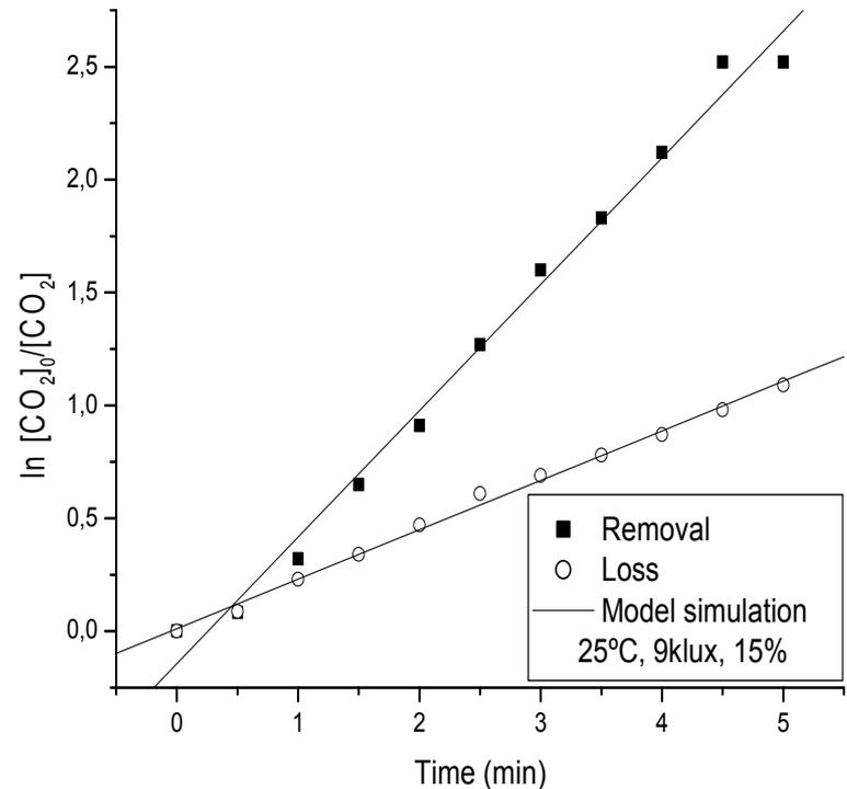
Fit of the experimental data by the integral method for the analysis of first order kinetic data
