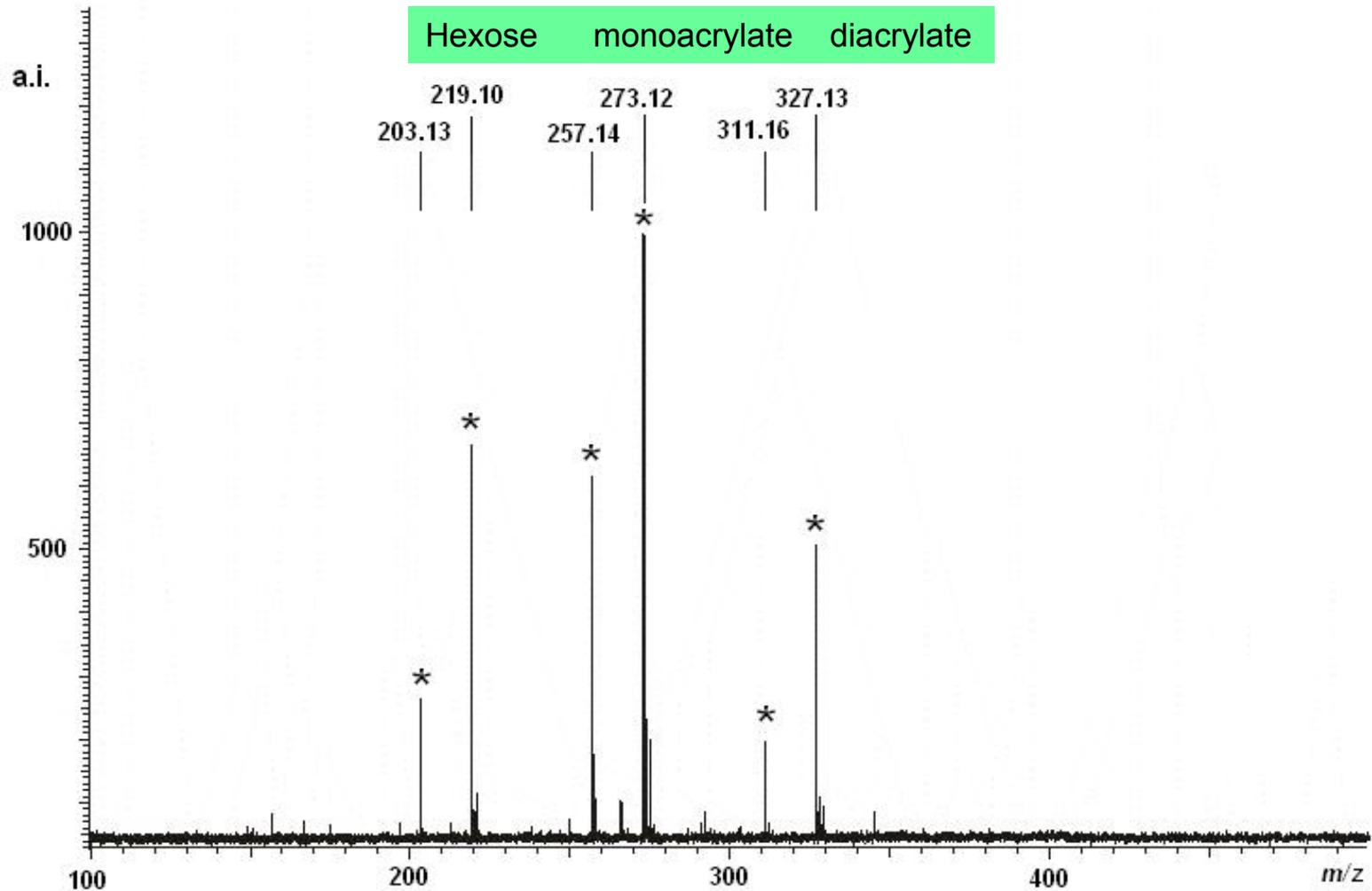
MALDI-TOF MS of the reaction mixtures of the lipase catalyzed esterifications of **D-fructose**, recorded after a reaction time of 48h. Asterisks indicate peaks from fructose and acrylates.
