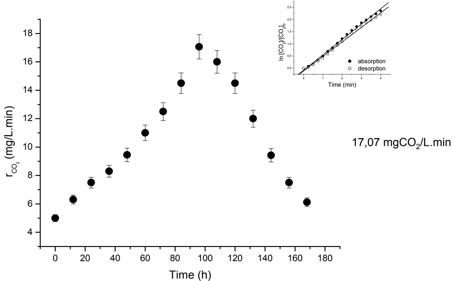
Carbon dioxide sequestration rates and fit of the experimental data by the integral method (measurements in the liquid phase)
