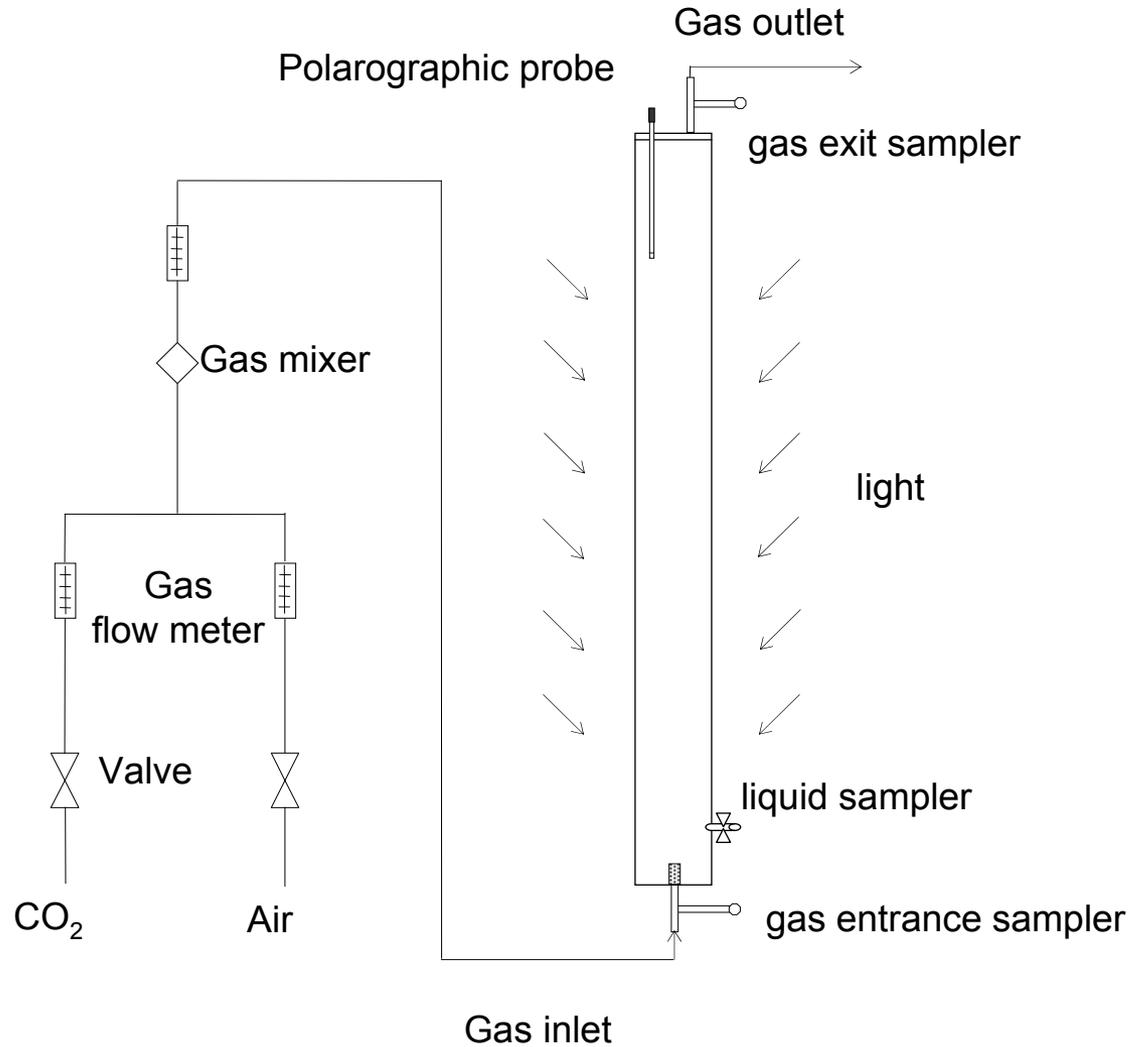
Schematic diagram of the photobioreactor
