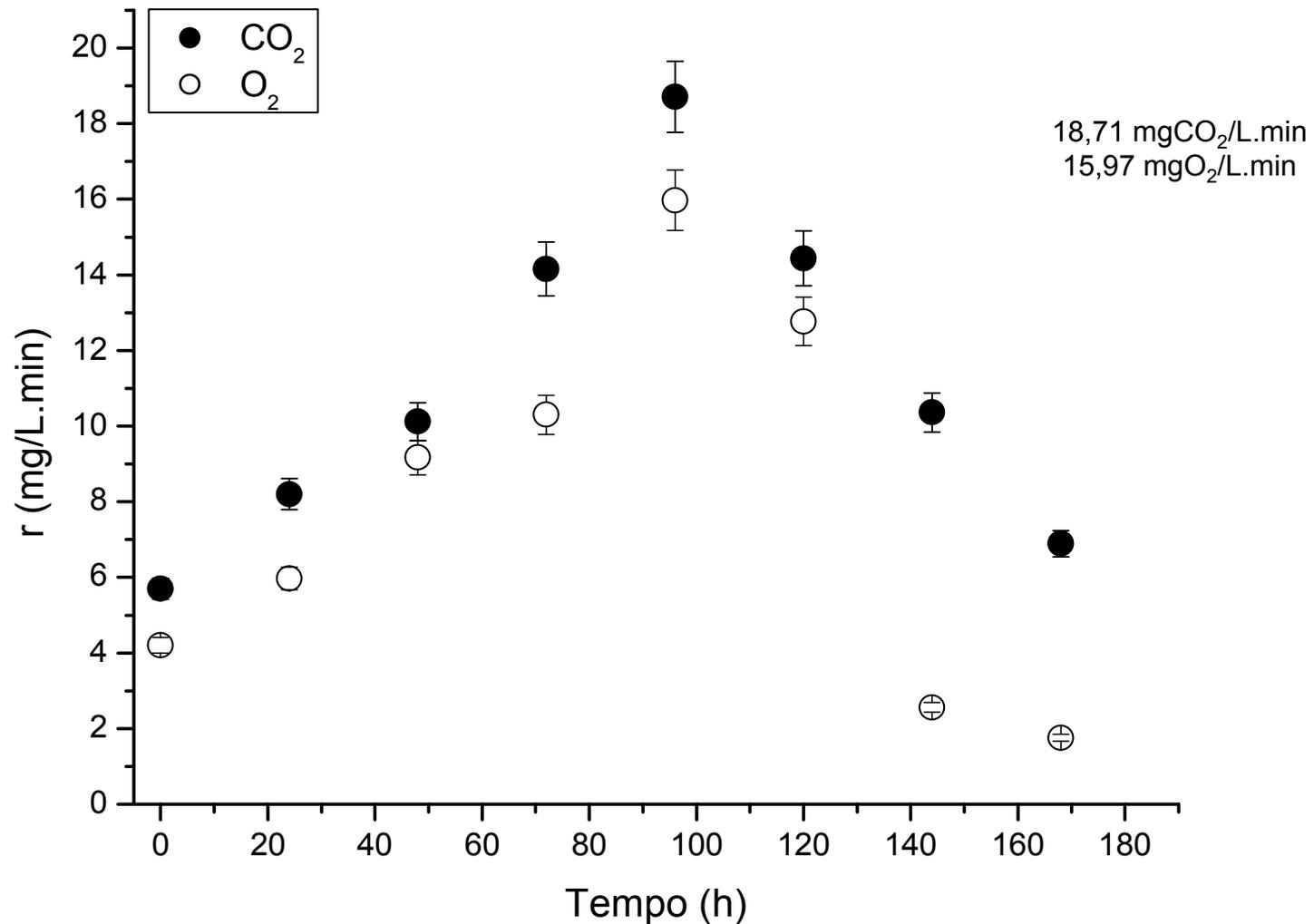
Figure 9: Carbon dioxide sequestration and oxygen release rates; ● CO<sub>2</sub> ○ O<sub>2</sub> (measurements in the gaseous phase)
