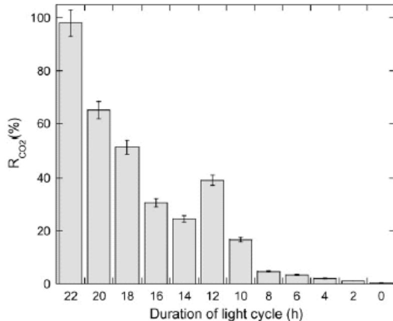
Percent carbon dioxide fixation rates (into biomass) as related to the duration of the light periods (bubble column reactor for optimized conditions).
