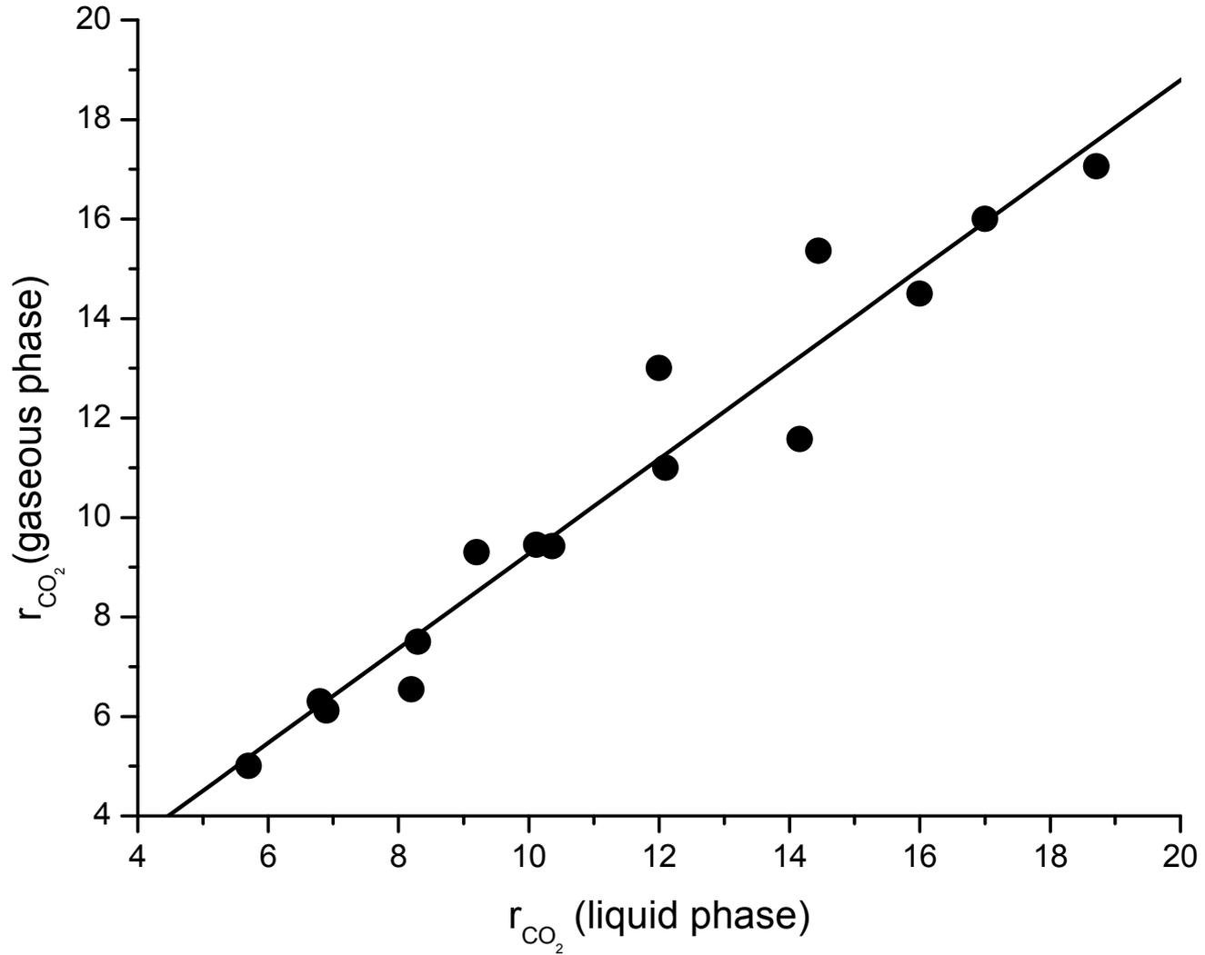
Comparison between carbon dioxide sequestration rates evaluated in the liquid and gaseous phases
