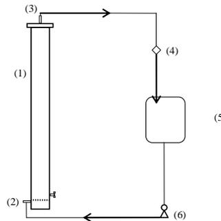
(C) BCR reactor with air recirculation
