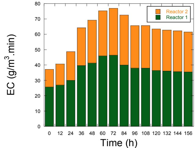
Kinetic data for two airlift reactors in series in the optimized conditions. Tested conditions: configuration (airlift); operational mode (simple operation, air recirculation and two reactors in series). EC: elimination capacity. RE: removal efficiency.
