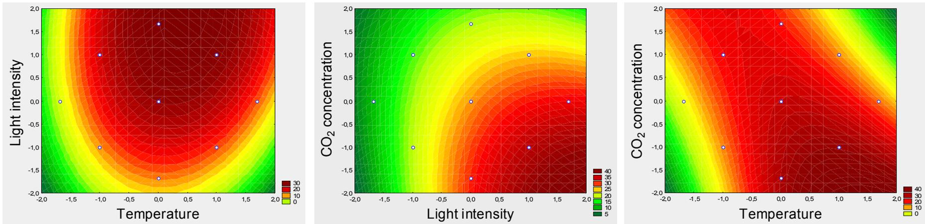
Figure 3: Contour curves for carbon fixation rate into biomass by the *Aphanothece microscopica* Nägeli (cultivations in bubble column reactor). Tested conditions: temperature (21, 25, 30, 35, 38°C); light intensity (0.96, 3, 6, 9, 11klux) and CO<sub>2</sub> concentration (3, 15, 25, 50, 62%).
