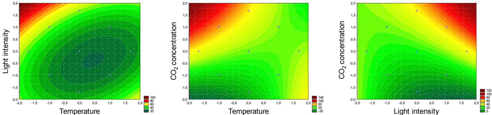
Contour curves for the variable carbon dioxide removal rate.
