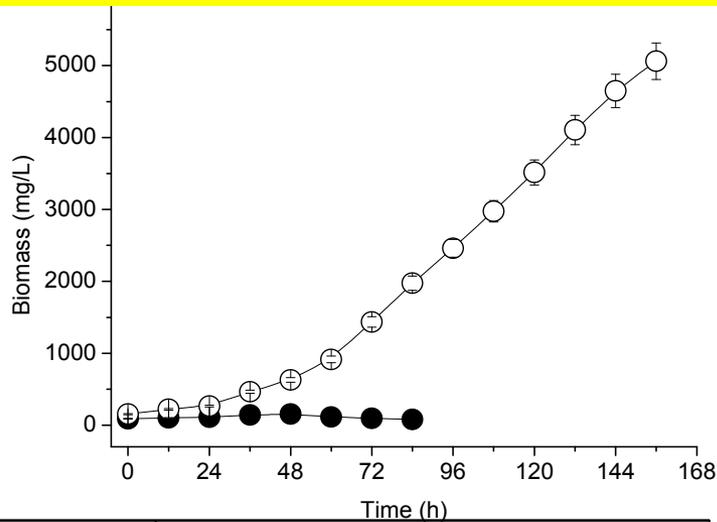
Growth curves in the refinery wastewater (closed symbols) and in the synthetic BGN medium (open symbols).
