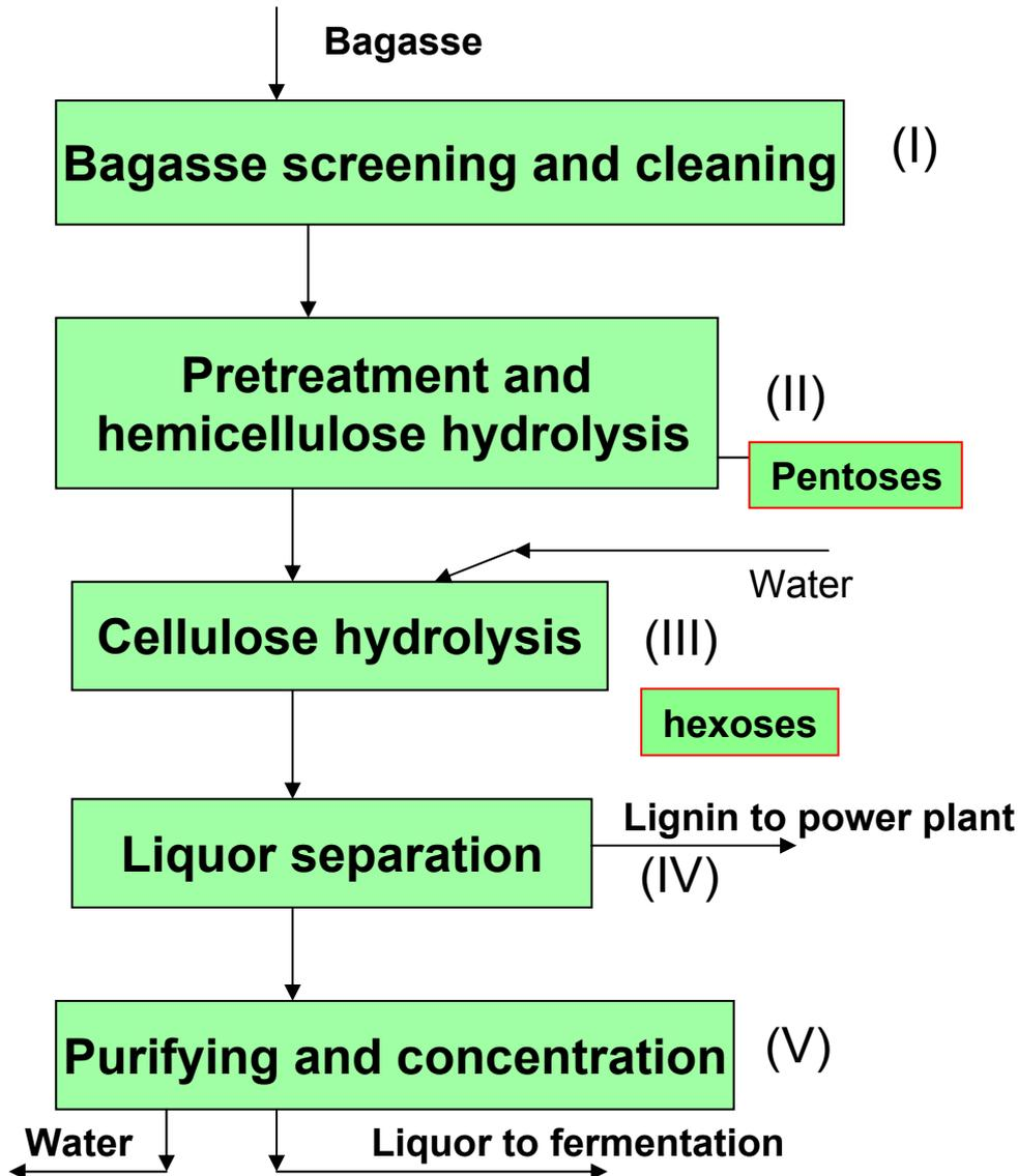
(I) Rind, pith and sand removed from fiber
