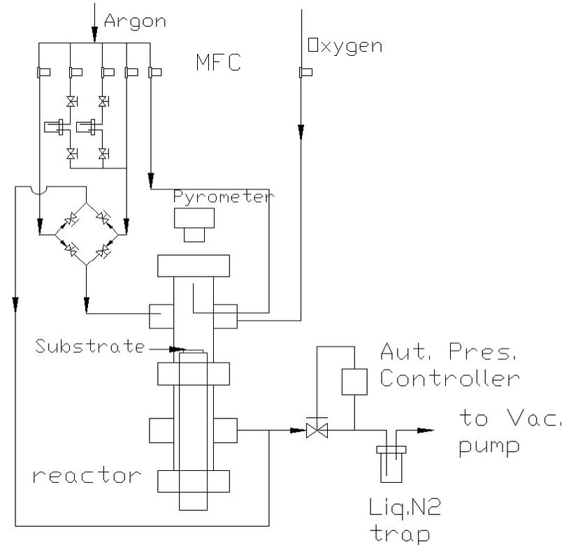
**Schematic of CVD testbed**
