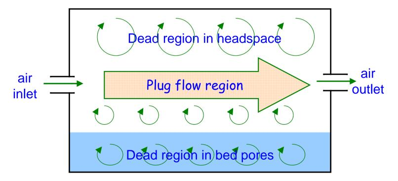
What do models and experimental results tell us about <u>rotating drum</u> type bioreactors...and what would we still like to know? (2) Gas flow patterns (cont'd)
