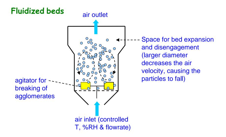
The air is blown at sufficient velocity to fluidize the substrate particles
