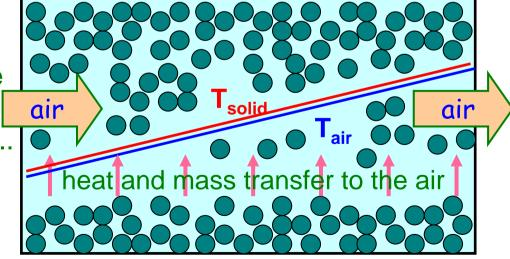
...with the 1 in T<sub>air</sub> its vapor-carrying capacity increases, so it removes water from the bed What do models and experimental results tell us about <u>packed-bed</u> type bioreactors....and what would we still like to know? (cont'd)
