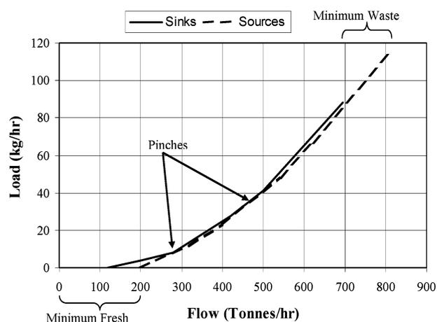
**Figure 10.** Shifted source/sink composite curves for example 1.**Table 2. Process Information for Example 2**
