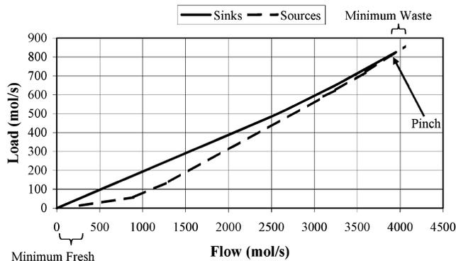
**Figure 14.** Shifted source/sink composite curves for example 4.
