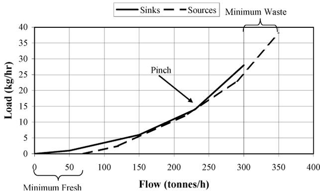
Figure 11. Shifted source/sink composite curves for example 2.
