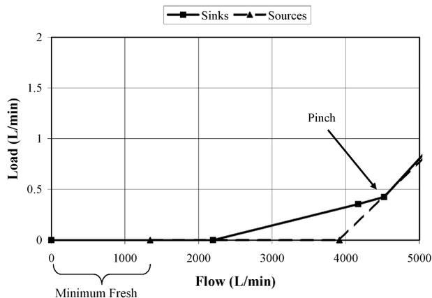
**Figure 13.** Magnified shifted source/sink composite curves for example 3.
