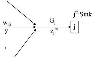
Figure 3. Mixing of sources at inlets of sinks.
